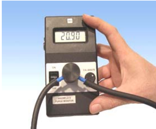
Weld Purge Monitor – Instrument de prelevare continua
