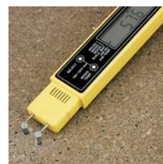
Concrete moisture contents
